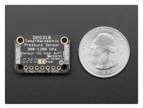
You can use this sensor with either I2C or SPI, so it's easy to integrate into projects. It also has a temperature sensor built in, with  $\pm$  0.5°C accuracy. For the lowest noise readings, set it up to take multiple measurements and perform a low-pass filter, that capability is built in! You can use it from 300 to 1200 hPa and in ambient temperature ranges from -40 to 85 °C.
